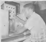
In the Instrument Section, electrical student Johnson Warner checks the function of an automatic distillation apparatus.
